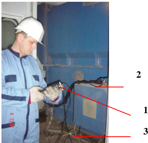
Figure 2 On line PD Detection: 1 – measuring Instrument; 2 – Frame Sensor (DIACS-TMP); 3 – CT Sensor (DIACS CT-68M).
